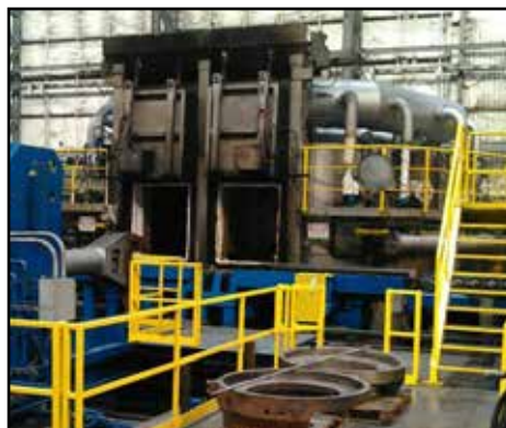
EXTRUSION PRESS LINE - INCLUDES: ROTARY HEARTH FURNACE, VERTICAL EXPANSION PRESS, PREHEAT INDUCTION UNITS, 7000 TON EXTRUSION PRESS
