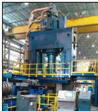
EXTRUSION PRESS LINE - INCLUDES: ROTARY HEARTH FURNACE, VERTICAL EXPANSION PRESS, PREHEAT INDUCTION UNITS, 7000 TON EXTRUSION PRESS
