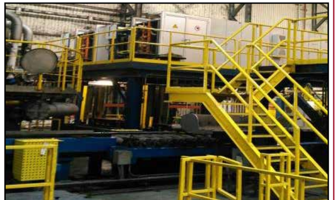
EXTRUSION PRESS LINE - INCLUDES: ROTARY HEARTH FURNACE, VERTICAL EXPANSION PRESS, PREHEAT INDUCTION UNITS, 7000 TON EXTRUSION PRESS
